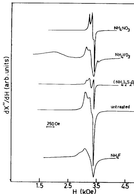
Fig. 3. Electron spin resonance spectra from the reaction products of  $\text{Ba}_3\text{SrCu}_2\text{O}_6 \cdot 2\text{CO}_2$  after grinding with various ammonium salts as indicated against the spectra.
