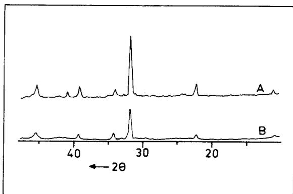
Fig. 2. X-ray diffraction patterns of  $\text{Ba}_3\text{SrCu}_2\text{O}_6$  (A) and the reaction product after grinding with ammonium fluoride (B).
