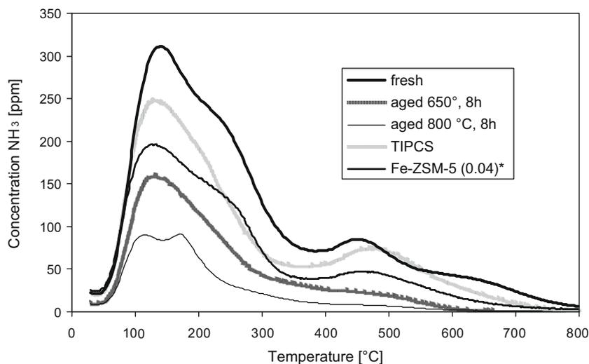
Fig. 7. Measured  $\text{NH}_3$  concentration during TPD of Fe-ZSM-5 (0.04)\* and Fe-ZSM-5 (0.3) in the fresh state, after silanization and after aging at 650 °C and 800 °C, respectively.
