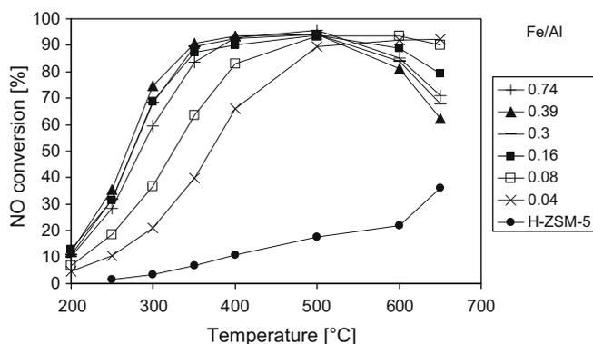
Fig. 4. NO reduction as a function of temperature over Fe-ZSM-5 catalysts with various exchange degrees (Fe/Al). Reaction conditions: 1000 ppm NO, 1000 ppm,  $\text{NH}_3$ , 10%  $\text{O}_2$ , 5%  $\text{H}_2\text{O}$ , remaining gas feed consists of  $\text{N}_2$ . GHSV = 52,000  $\text{h}^{-1}$ .
