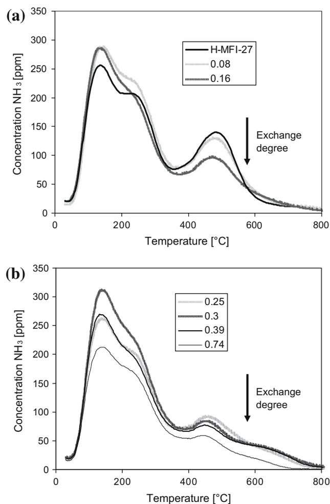
Fig. 1. Measured  $\text{NH}_3$  concentration during TPD for (a) H-ZSM-5 and Fe-ZSM-5 (0.08, 0.16) and (b) Fe-ZSM-5 (0.25, 0.3, 0.39, and 0.74).
