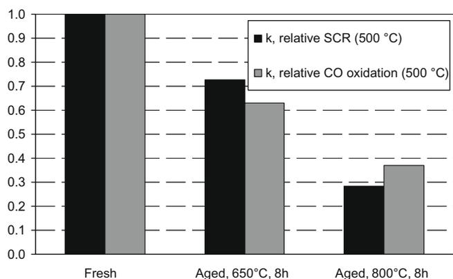
Fig. 11. CO oxidation activity at 500 °C and relative first-order rate constants for the standard SCR reaction at 500 °C for fresh and 650 °C and 800 °C aged Fe-ZSM-5 (0.3).
