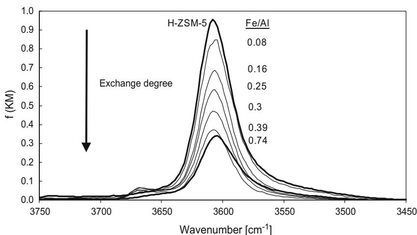
Fig. 2. FTIR spectra of the hydroxyl stretching region for Fe-ZSM-5 samples with various exchange degrees.
