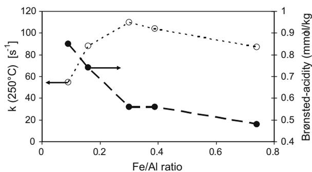
Fig. 5. First-order rate constants for the SCR reaction and Brønsted acidity as a function of the exchange degree.
