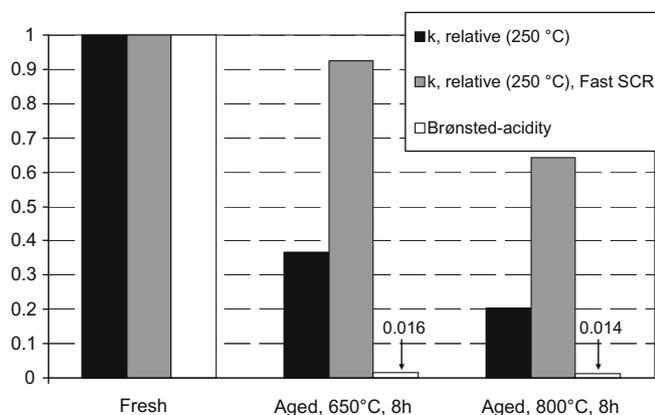
Fig. 10. Relative Brønsted acidity and relative first-order rate constants for the standard SCR reaction and fast SCR reaction, calculated from Fig. 9 for fresh and 650 °C and 800 °C aged Fe-ZSM-5 (0.3).
