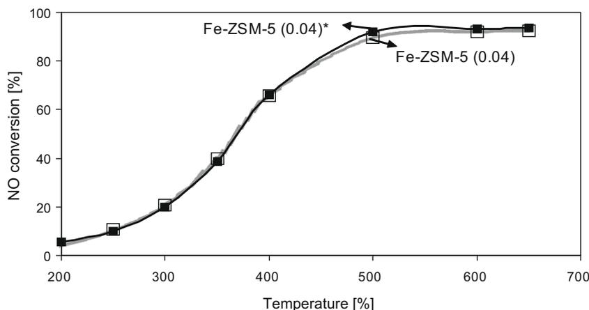
Fig. 6. NO reduction as a function of temperature over two Fe-ZSM-5 samples with equal exchange degree (Fe/Al = 0.04), but with different Brønsted acidities: Fe-ZSM-5 (0.04) 89% and Fe-ZSM-5 (0.04)\* 22% relative to the acidity of the parent H-ZSM-5. Reaction conditions: 1000 ppm NO, 1000 ppm,  $\text{NH}_3$ , 10%  $\text{O}_2$ , 5%  $\text{H}_2\text{O}$ , remaining gas feed consists of  $\text{N}_2$ . GHSV = 52,000  $\text{h}^{-1}$ .
