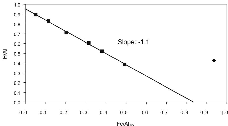
Fig. 3. Change of  $\text{H}/\text{Al}$  ratio with  $\text{Fe}/\text{Al}_{\text{av}}$  ratio for Fe-ZSM-5 samples with various exchange degrees, with  $\text{Al}_{\text{av}}$  corresponding to the concentration of available Brønsted acid sites determined in Table 1.
