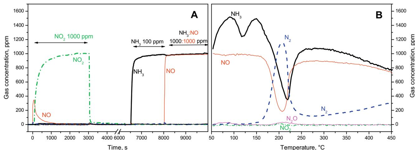
**Fig. 2.** (A) TRM at 50 °C: NO<sub>2</sub> adsorption (1000 ppm) and nitrates + NH<sub>3</sub> (1000 ppm) + NO (1000 ppm) in a flow of H<sub>2</sub>O = 1%, O<sub>2</sub> = 0%, He balance; (B) TPSR: T-ramp at 20 K/min while flowing NH<sub>3</sub> (1000 ppm) + NO (1000 ppm), H<sub>2</sub>O = 1%, O<sub>2</sub> = 0%, He balance.
