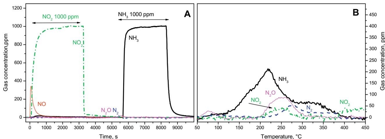
**Fig. 4.** (A) TRM at 50 °C:  $\text{NO}_2$  adsorption (1000 ppm) followed by  $\text{NH}_3$  adsorption (1000 ppm) in a flow of  $\text{H}_2\text{O} = 1\%$ ,  $\text{O}_2 = 0\%$ , He balance; (B) TPD: T-ramp at 20 K/min while flowing He +  $\text{H}_2\text{O} = 1\%$ .
