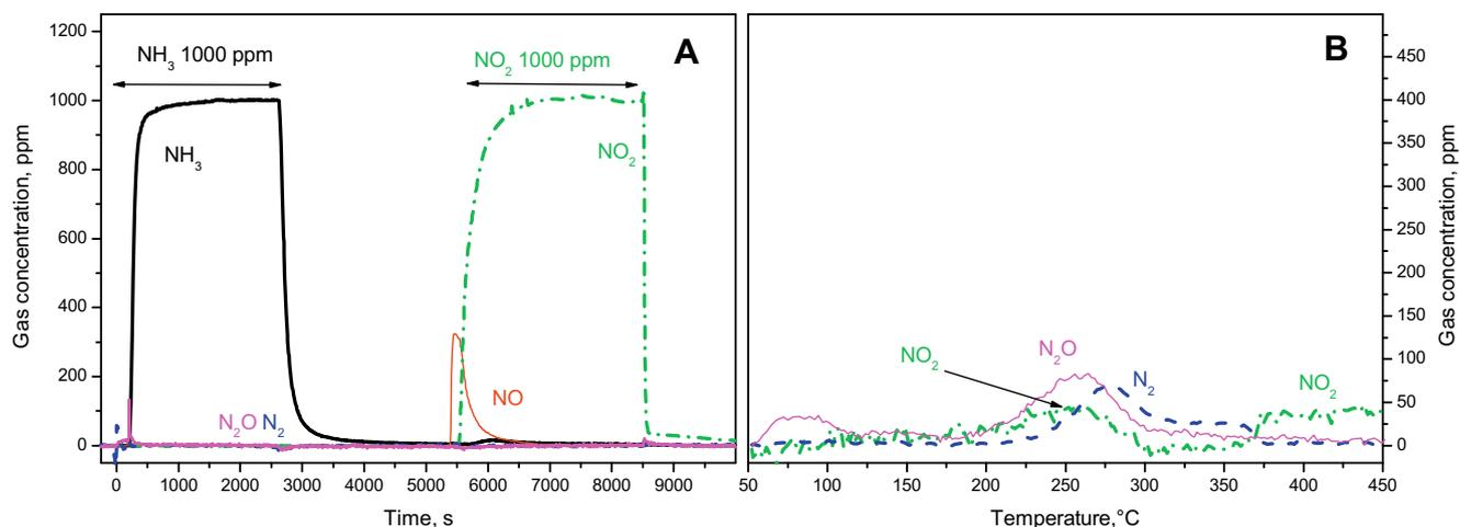
**Fig. 3.** (A) TRM at 50 °C:  $\text{NH}_3$  adsorption (1000 ppm) followed by  $\text{NO}_2$  adsorption (1000 ppm) in a flow of  $\text{H}_2\text{O} = 1\%$ ,  $\text{O}_2 = 0\%$ , He balance; (B) TPD: T-ramp at 20 K/min while flowing He +  $\text{H}_2\text{O} = 1\%$ .
