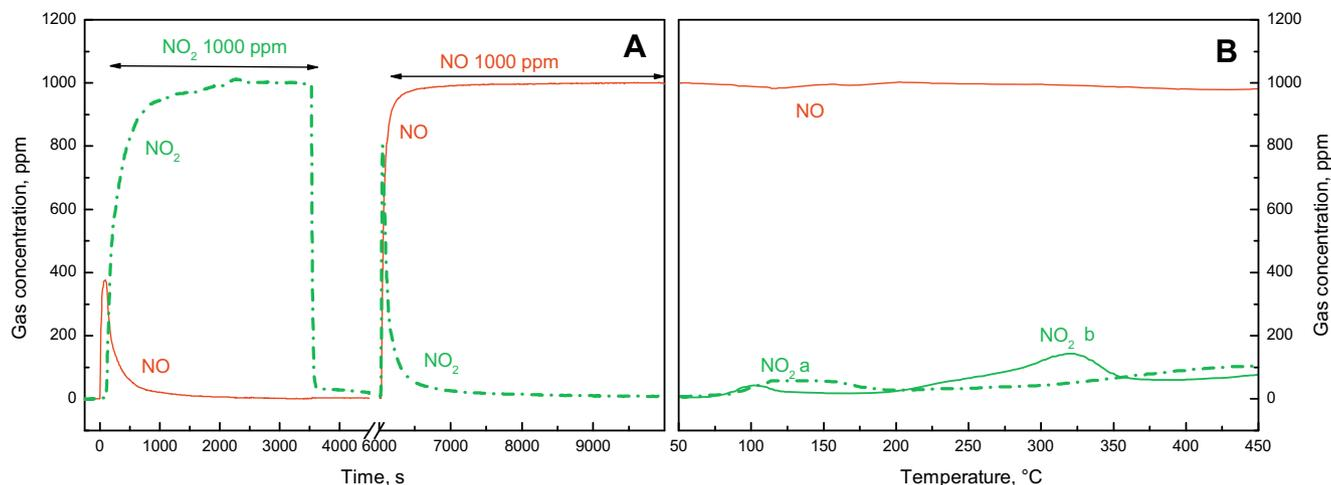
**Fig. 1.** (A) TRM at 50 °C: NO<sub>2</sub> adsorption (1000 ppm) followed by nitrates + NO (1000 ppm) reaction in a flow of H<sub>2</sub>O = 1%, O<sub>2</sub> = 0%, He balance; (B) TPSR: T-ramp at 20 K/min while flowing NO (1000 ppm), H<sub>2</sub>O = 1%, O<sub>2</sub> = 0%, He balance. Curve b in (B) is the NO<sub>2</sub> trace from a TPD run (thermal decomposition in inert atmosphere of nitrates formed by NO<sub>2</sub> adsorption at 50 °C, T-ramp at 20 K/min).
