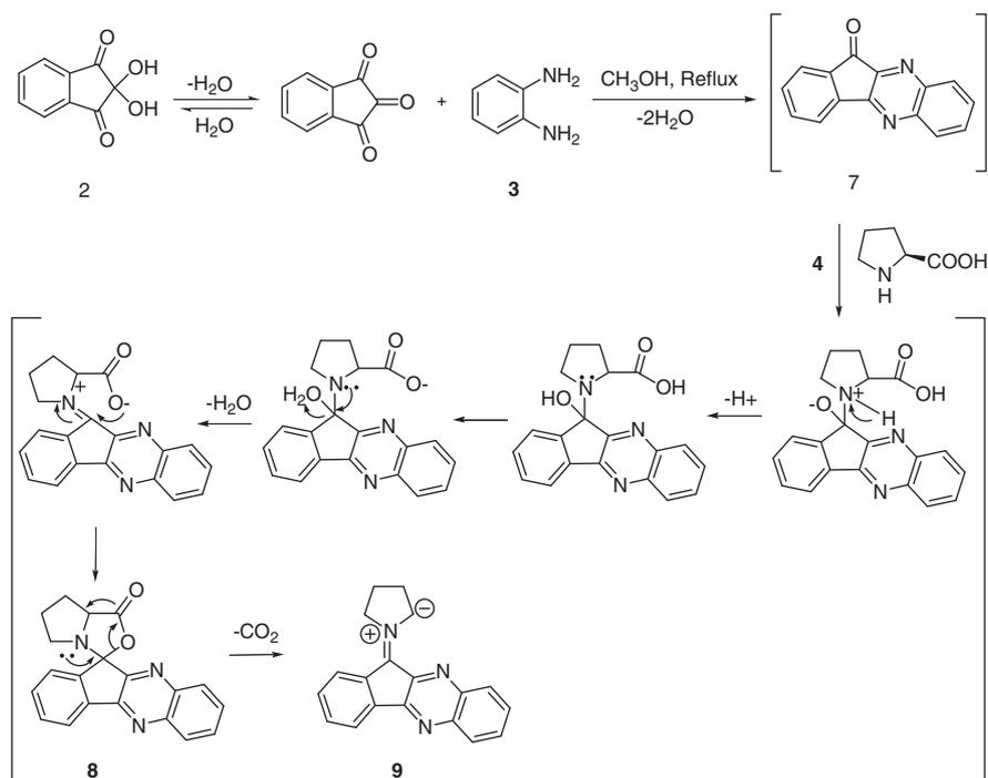
**Figure 1.** Mechanism for the formation of azomethine ylide **9** from ninhydrin **2**, 1,2-phenylenediammine **3**, and L-proline **4**.
