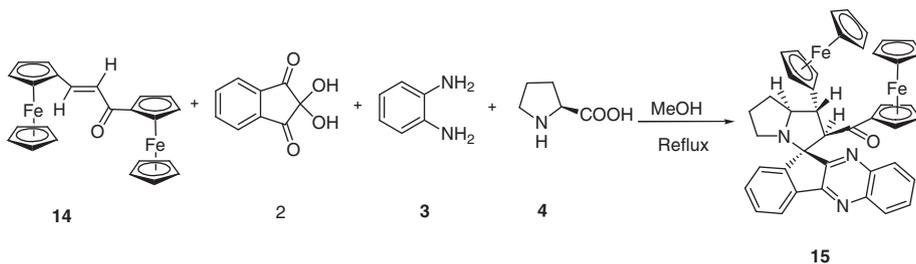
**Scheme 4.** Synthesis of ferrocene grafted spiro-indenoquinoxaline ferrocenyl pyrrolizidine **15**.
