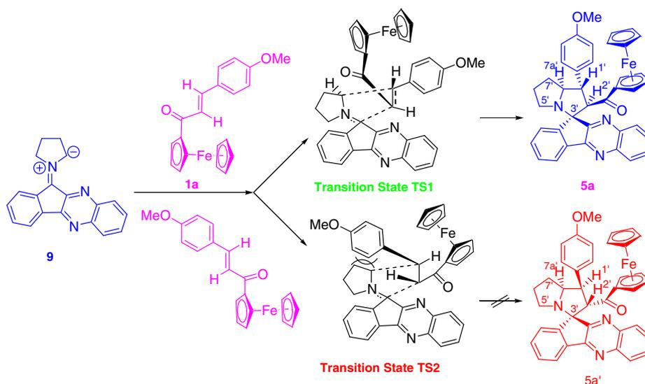
**Figure 2.** The proposed mechanism for one-pot four-component synthesis of ferrocene grafted spiro-indenoquinoxaline-pyrrolizidine **5**.
