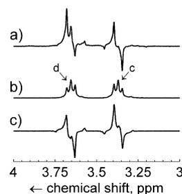
**Figure 2.** <sup>1</sup>H NMR spectra observed immediately after bubbling the produced ethylene through the PTSC solution (a,c) and 20 s after the bubbling was stopped (b). The spectrum in (c) was acquired using double-quantum filtering. The signal labels in (b) refer to the adduct structure in Figure 1.
