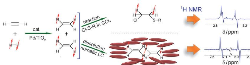
**Taking CH<sub>2</sub>CH<sub>2</sub> for a spin:** Enrichment of the nuclear spin isomers of ethylene was achieved by catalytically reacting acetylene with parahydrogen (see scheme). The spin isomers were used for NMR signal enhancement, both with and with-
