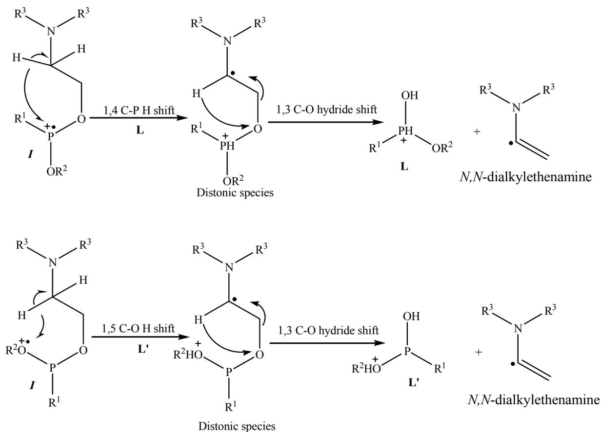
Figure 5. Proposed mechanisms for formation of ion [L].
