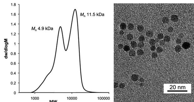
**Fig. 3** Left: GPC trace for polymer **4** in chloroform, calibrated against PEG standards; the two peaks correspond to single-length and double-length chains arising from association via the “Roman Handshake”. Right: transmission electron micrograph showing micellar nanoparticles of polymer **4** on a graphene oxide support.
