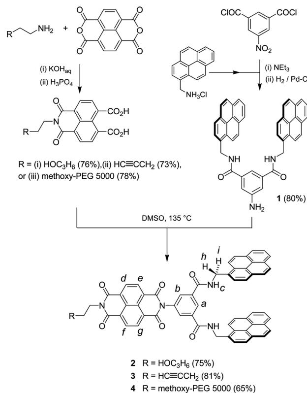
**Scheme 1** Synthesis of the amino-functional tweezer-molecule **1**, the self-complementary imido-tweezers **2** and **3**, and the corresponding tweezer-end-capped polymer **4**.
