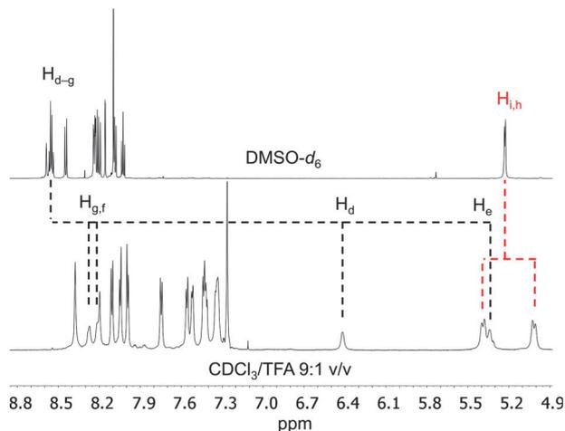
**Fig. 1** Comparative  $^1\text{H}$  NMR spectra of **3** ( $\text{R} = \text{CH}_2\text{C}\equiv\text{CH}$ ) in  $\text{d}_6$ -DMSO and  $\text{CDCl}_3/\text{TFA}$  (9 : 1 v/v). Note the very large self-complexation-induced resonance shifts and magnetic inequivalencies for protons  $\text{H}^d$  and  $\text{H}^e$  in the spectrum when  $\text{CDCl}_3/\text{TFA}$  is used as solvent.
