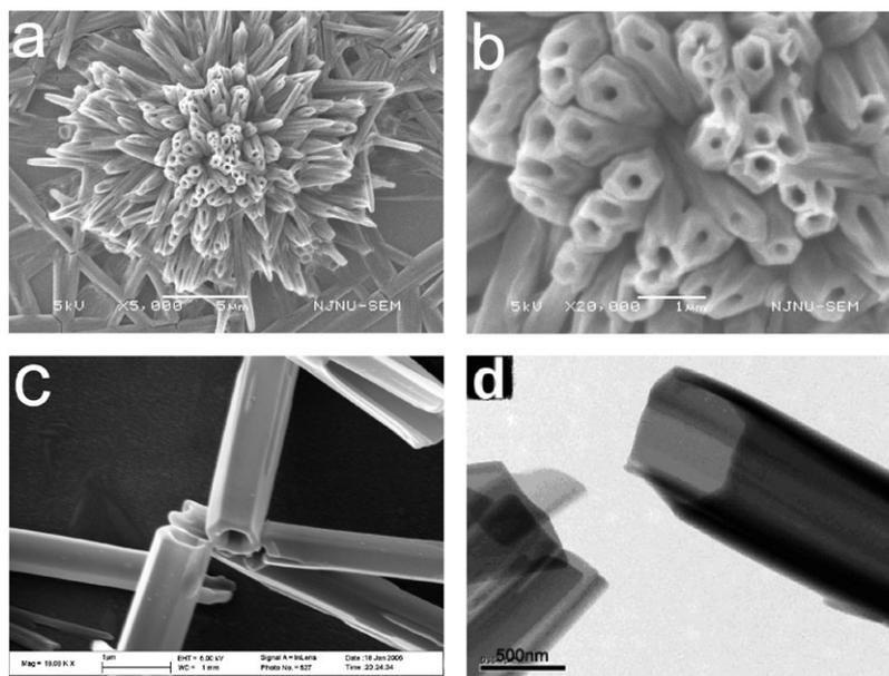
**Fig. 6** (a) SEM image of the product from crystallization of a drop of TMPTA THF solution on a glass slide, (b) enlarged view of (a), (c) SEM image of the tubule obtained by the reprecipitation method, (d) corresponding TEM image of the tubule obtained by the reprecipitation method.
