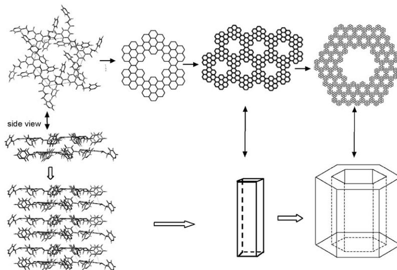
**Fig. 5** Proposed formation process of the hexagonal microtubes. This scheme describes the assembly mode of the moieties in the hexagonal microtube, and it doesn't show the definite diameter of the microtube.
