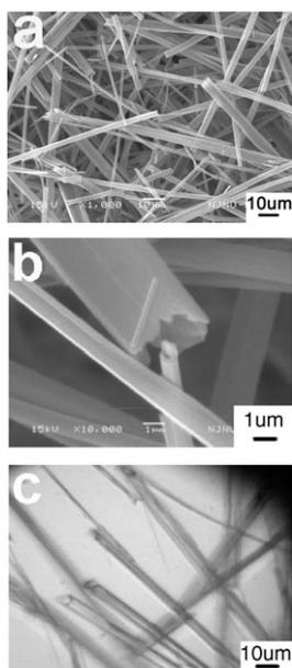
**Fig. 1** (a) SEM image of the microtubes obtained in solvent of  $\text{H}_2\text{O}$ -THF = 5 : 1 (v/v, 1.36 wt%), (b) higher magnification of (a), (c) corresponding optical microscopy image ( $\times 400$ ).
