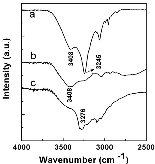
**Fig. 4** FT-IR spectra of (a) TMPTA hexagonal microtubes obtained in  $\text{H}_2\text{O}-\text{THF} = 5 : 1$  (v/v), (b) protonated TMPTA, (c) TPTA hexagonal crystals.
