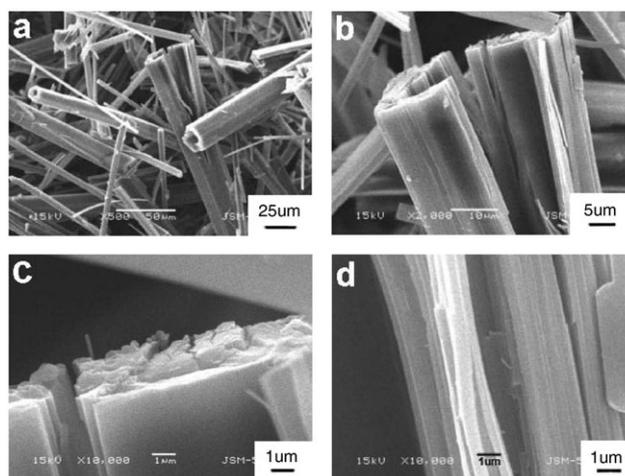
**Fig. 3** SEM images of the hexagonal microtubes obtained in the solvent of  $\text{H}_2\text{O}$ -THF = 3 : 1 (v/v) at higher concentration of 2.0 wt% (a) corresponding low magnification image, (b) enlarged view of the broken tube, (c) higher magnification of the cross-section face of the broken tube, (d) higher magnification of the fractured face of the broken tube.
