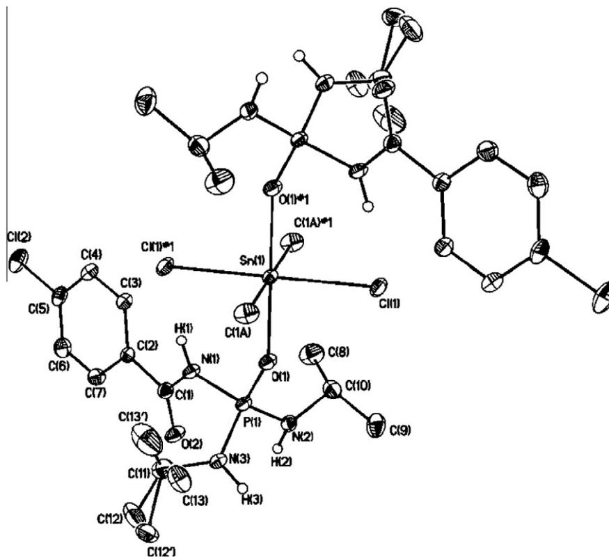
Fig. 11. Molecular structure and atom-labeling scheme for complex **8** (50% probability ellipsoids).
