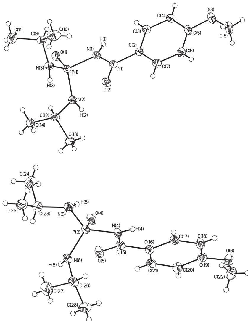
**Fig. 1.** Molecular structure and atom-labeling scheme for **2** (40% probability ellipsoids).
