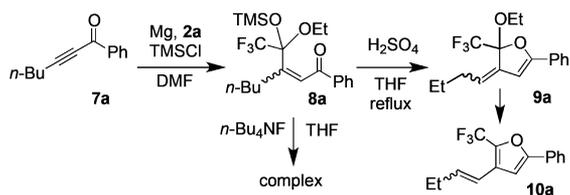
investigation of the cyclization reaction conditions (see Table S2), **8a** could be selectively converted to (*E*)-2-trifluoromethylated furan **10a** with the aid of sulfuric acid in THF under reflux conditions. A variety of trifluoromethylated furans **10** were synthesized, and the results are shown in Scheme 4. Significant
