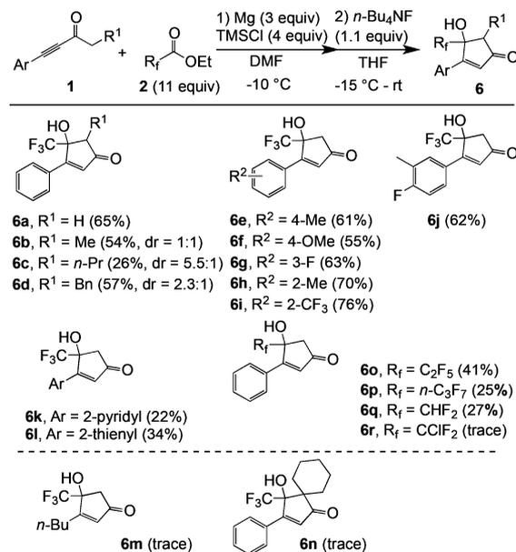
of the phenyl ring slightly decreased the yields (**6e** and **6f**), and that at the *ortho*-position exhibited the increase of yields (**6h**). Substitution by a fluorine atom at *meta*-position afforded **6g** in 63% yield, and a strong electron-withdrawing trifluoromethyl group at the *ortho*-position gave the desired product **6i** in 76% yield.
