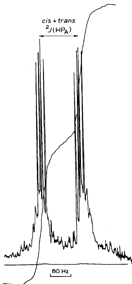
Fig. 3. ^1\text{H} NMR spectrum of [\text{Ir H}_2\text{P}(\text{O})(\text{OMe})_2(\text{P}(\text{OMe})_3)_3] , hydride region.
