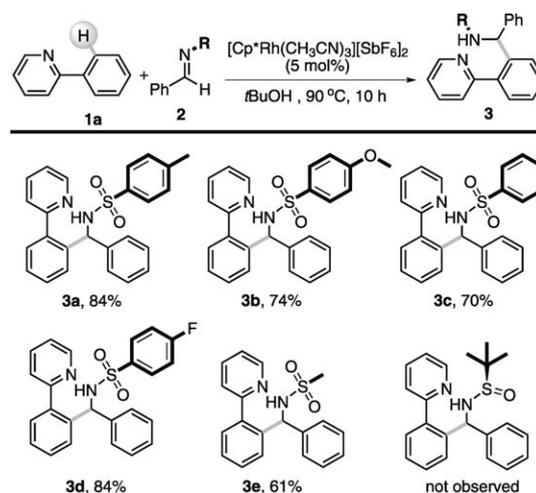
**Scheme 2.** Addition of the C–H bond of **1a** to different benzaldimines **2**. Reaction conditions: **1a** (0.25 mmol), **2** (0.50 mmol), *t*BuOH (1.0 mL). The yield of isolated product is reported.
