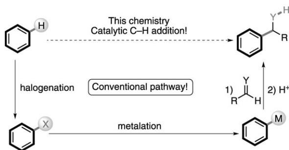
**Scheme 1.** Rational design of direct C–H addition toward C=Y. Conventional arylation of C=Y through halogenations/metalation/nucleophilic addition-hydration sequence versus “ideal” direct C–H addition to C=Y, where Y = N or O. X = halogen.
