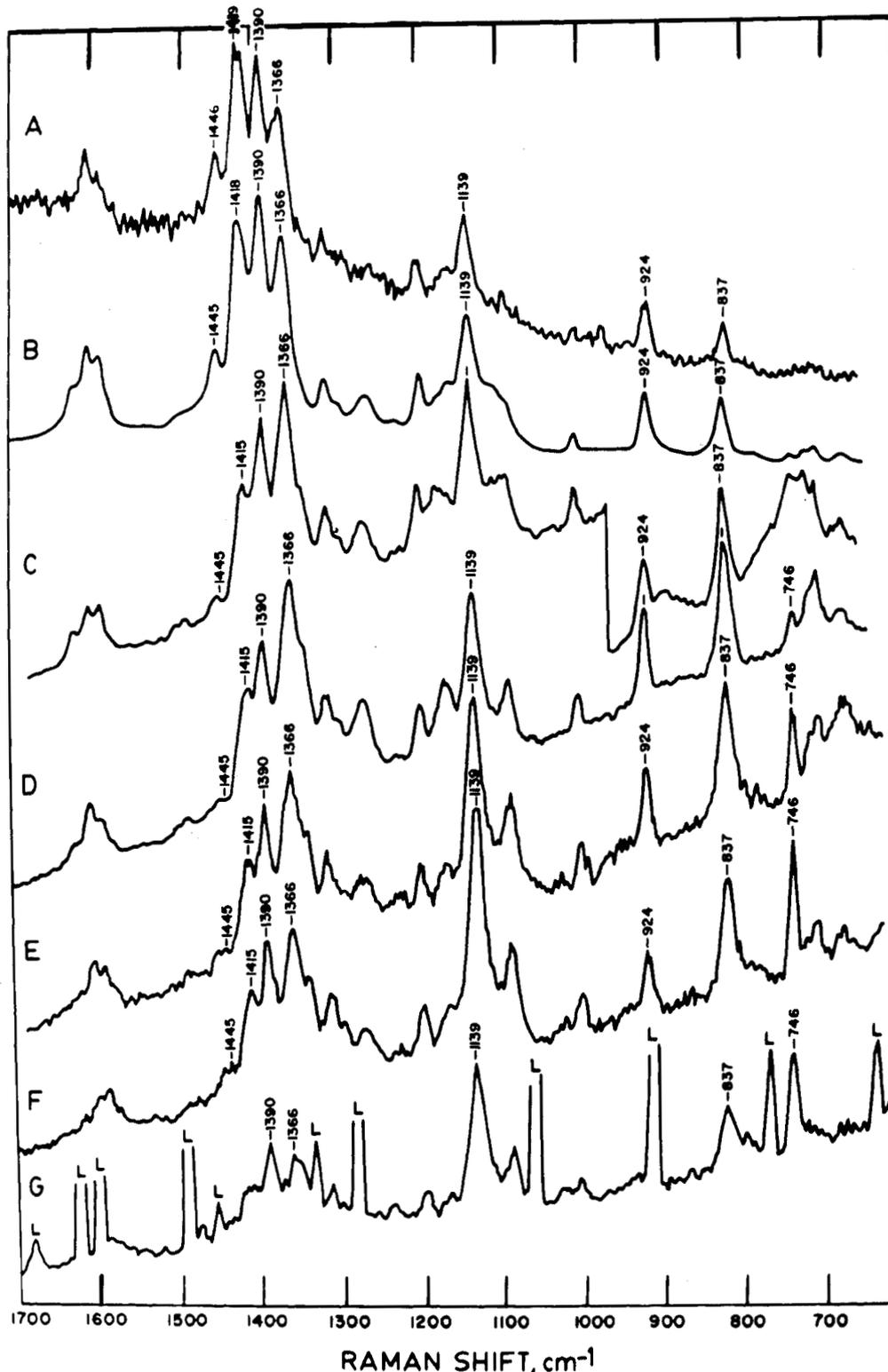
**Figure 3.** Raman spectra: A,  $1.3 \times 10^{-4}$  M DABS-ASP,  $\lambda_0 = 465.8$  nm; B, C, D, sol 6 with  $4 \times 10^{-7}$  M DABS-ASP (total concentration),  $\lambda_0 = 488.0, 572.5, 591.5$  nm, respectively; E, F, G, sol 6 with  $1.1 \times 10^{-5}$  M DABS-ASP (total concentration),  $\lambda_0 = 624.7, 647.1, 676.4$  nm, respectively. Laser plasma lines in G are denoted L.
