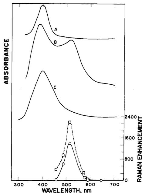
**Figure 2.** Absorption spectra of A, silver citrate hydrosol, centrifuged sol 3; B, sol 6 with DABS-ASP; C, Sol 3 with DABS-ASP. SERS excitation profiles, absolute surface enhancement for sol 3, solid line; lower limit of enhancement for sol 6, dashed line.
