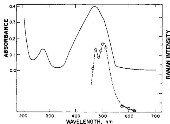
Figure 1. Absorption spectrum of DABS-ASP ( $1.08 \times 10^{-4}$  M) in 0.01 M Na<sub>2</sub>Cit, solid line; resonance Raman excitation profile of DABS-ASP ( $1.08 \times 10^{-4}$  M) vs. Na<sub>2</sub>SO<sub>4</sub> (0.9 M) internal standard,  $I_{\text{DABS-ASP}} (\sim 1400 \text{ cm}^{-1})/I_{\text{SO}_4^{2-}} (985 \text{ cm}^{-1})$ , dashed line.
