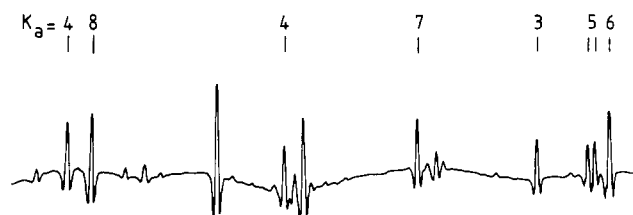
Figure 2. Part of the HCSCN spectrum showing a characteristic pattern with different K a components of the J :33←32 transition (together with some lines belonging to an unidentified byproduct); frequency scan 204.2–204.3 GHz.
