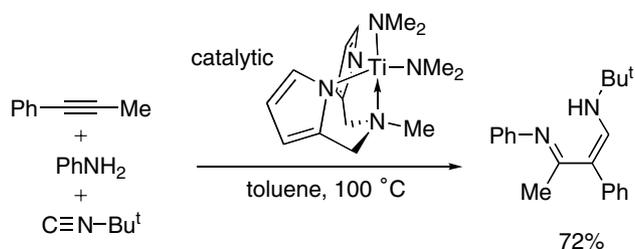
Scheme 1. Example of iminoamination catalyzed by a titanium pyrrolyl complex.
