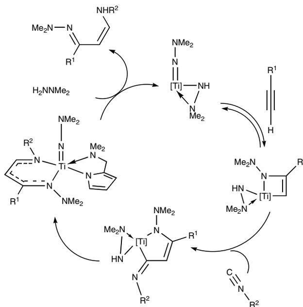
Scheme 6. Working model for imino-hydrazination catalyzed by **1**. [Ti] =  $\text{Ti}(\text{dap})$ .
