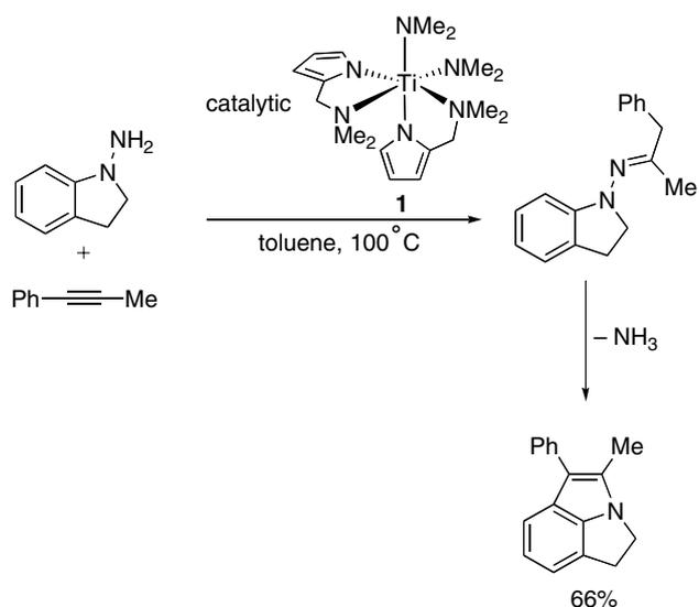
Scheme 2. Hydrohydrazination of an alkyne catalyzed by **1** and Fischer cyclization.
