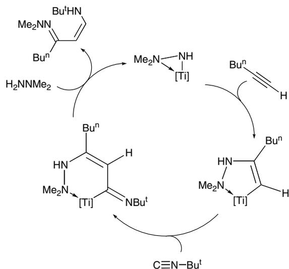
Scheme 4. Possible 1,2-insertion mechanism for iminohydrazination.
