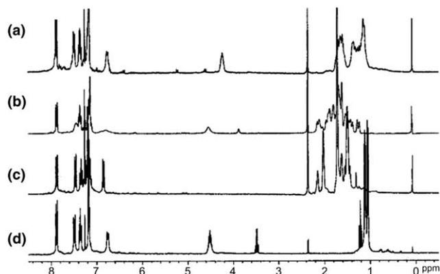
Chart 2. (a) Ti(BINOLato)(O-cyclohexyl)<sub>2</sub> (**8**); (b) Ti(BINOLato)(O-2-adamantyl)<sub>2</sub> (**11**); (c) Ti(BINOLato)(O-1-adamantyl)<sub>2</sub> (**10**); (d) Ti(BINOLato)(OPr<sup>i</sup>)<sub>2</sub> (**1**).
