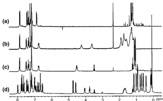
Chart 1. (a)  $\text{Ti}(\text{BINOLato})(\text{O}-t\text{-Bu})_2$  (**7**); (b)  $\text{Ti}(\text{BINOLato})(\text{O-cyclohexyl})_2$  (**8**); (c)  $\text{Ti}(\text{BINOLato})(\text{OPr}^i)_2$  (**1**); (d)  $\text{Ti}(\text{BINOLato})(\text{O-2,4-dimethyl-3-pentyl})_2$  (**9**).
