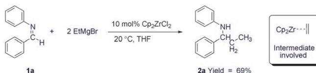
Scheme 1. Ethylation of aldimine **1a** catalyzed by [Cp<sub>2</sub>ZrCl<sub>2</sub>] (Cp = cyclopentadienyl).<sup>[13b]</sup>
