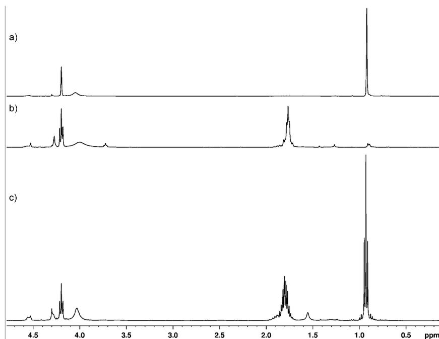
Figure 3. Comparison of the  $^1\text{H}$  NMR spectra of the products that arise from the reaction of a)  $\text{CH}_3\text{CD}_2\text{MgBr}$ , b)  $\text{CD}_3\text{CH}_2\text{MgBr}$ , and c)  $\text{CH}_3\text{CH}_2\text{MgBr}$  with **1a** in the presence of catalytic amounts of titanium isopropoxide.
