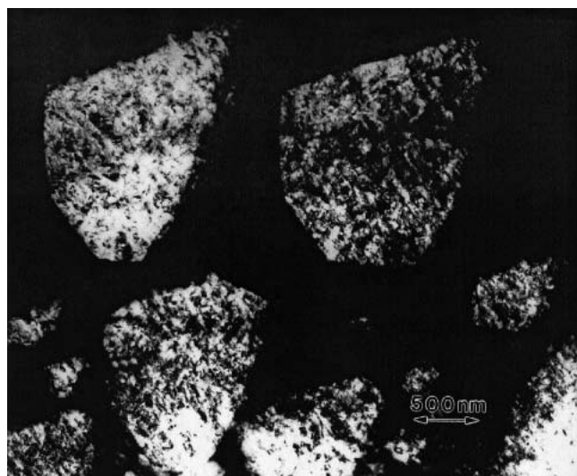
FIG. 6. Plan-view bright-field TEM image of pores in a CoGa grain covered by a \beta -Ga 2 O 3 scale. Scale grown during 24 h at 800 °C in air. Note the different pore sizes and the most similar pore shapes.
