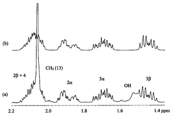
**Figure 3.** CH<sub>2</sub>(2)–CH<sub>2</sub>(3)–CH(4) signals of the 300 MHz <sup>1</sup>H NMR spectrum of **3** in CDCl<sub>3</sub>: (a) experimental; (b) calculated.
