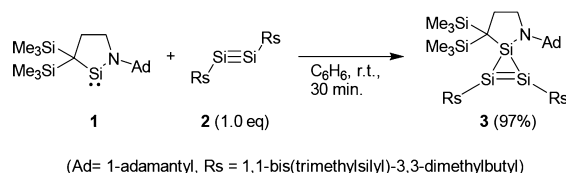
Scheme 1. [1 + 2] Cycloaddition of Silylene 1 and Disilyne 2
