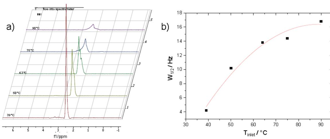
Figure 3 a) Stacked spectra of DMSO at different continuous flow temperature and
