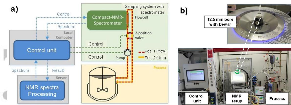
Figure 4 a) Schematic drawing of the process NMR system. Sampling system and the NMR spectrometer must be installed in vicinity to the respective process, control and spectra processing computers are connected via Ethernet and are stored in a watchdog folder. b) Photograph of the test assembly in a hood and photograph of the prototype NMR probe with Dewar for heated samples.
