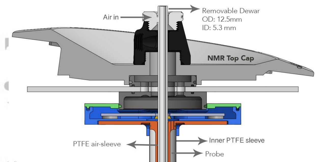
Figure 1 Sketch of the upper part of the prototype NMRReady with air sleeve and removable Dewar
