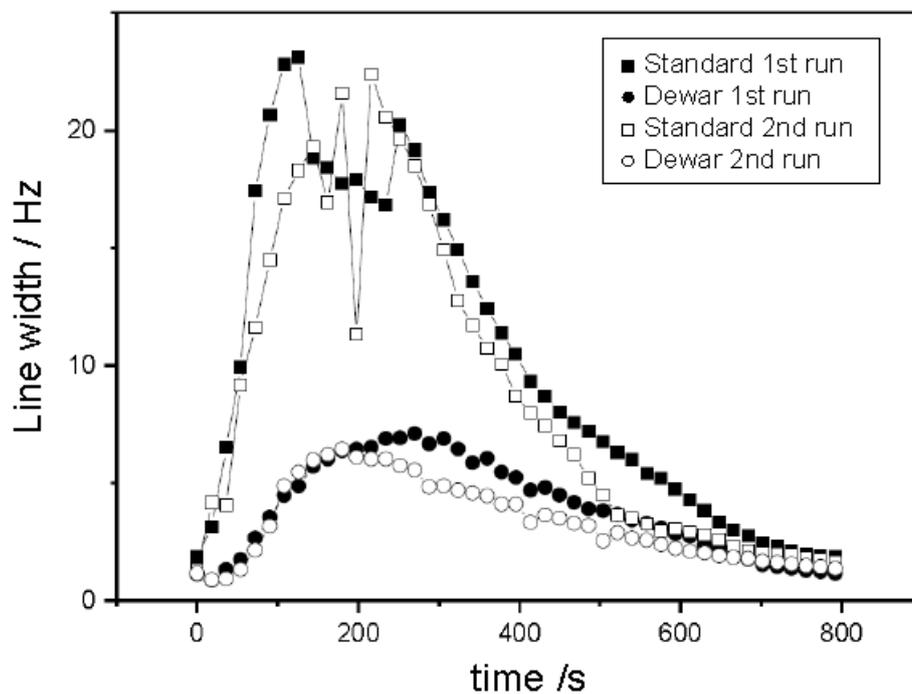
Figure 2 Water line width as determined by the by internal shimming of the NMR instruments as a function of time after 1 min exposure to an octanol sample preheated to 100°C. Square symbols: standard instrument, round symbols: prototype with Dewar
