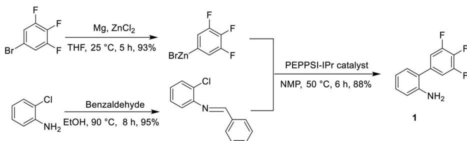
**Scheme 1.** Synthesis of compound **1** based on a Negishi coupling reaction.<sup>7</sup>
