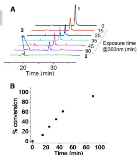
**Figure 1.** A HPLC profiles of a 0.5 mM solution of **1** in water at different exposure time at 360 nm ( $2.7$  mW/cm<sup>2</sup>). Elugrams were recorded with 210 nm channel in HPLC. B Conversion degree of the photolysis of **1**.
