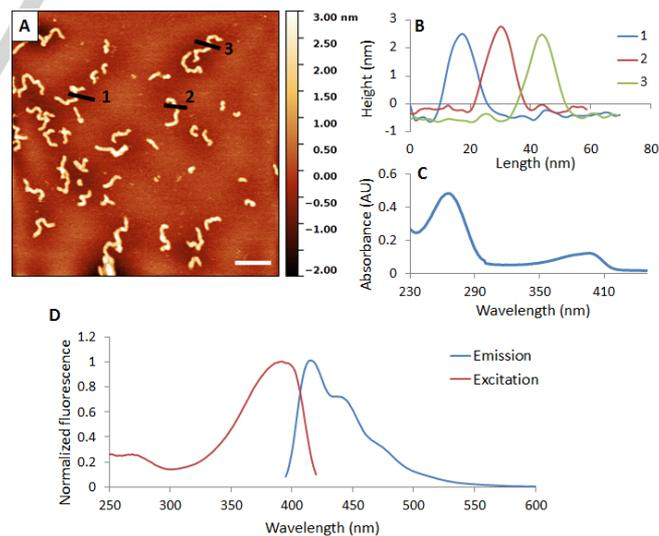
**Figure 1.** Characterization of **poly(F-DNA)**. **A)** Topography AFM image of a fraction containing medium size **poly(F-DNA)** carrying a 10mer DNA sequence. Scale bar = 100 nm. **B)** Height profile for **poly(F-DNA)** showing heights between 2 and 3 nm. **C)** UV-vis absorption spectrum for **poly(F-DNA)** carrying 15T oligonucleotides. **D)** Excitation (red line,  $\lambda(\text{em}) = 430$  nm) and emission (blue line,  $\lambda(\text{exc}) = 385$  nm) spectra for **poly(F-DNA)**.
