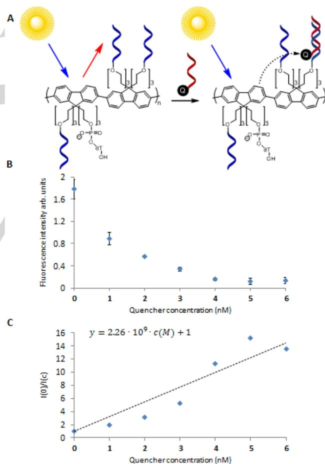
**Figure 4.** Quenching studies with **poly(F-DNA)**. **A)** Illustration of **poly(F-DNA)** binding to a complementary DNA strand carrying a dabcyil quencher. **B)** Data from titration with complementary quencher strand. 50 nM (5 pmol) of DNA on **poly(F-DNA)** was utilized in the experiments. Error bars denote 1 standard deviation from the mean derived from triplicates **C)** Stern-Volmer plot from the titration data.
