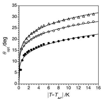
**Fig. 3** Optical tilt angles  $\theta_{\text{opt}}$  versus reduced temperature  $T - T_{\text{AC}}$  for compounds **1** (●), **2** (○) and **3** (△). The solid lines represent the fits to eqn (2) (**1**:  $\beta = 0.22$ ,  $R^2 = 0.947$ ; **2**:  $\beta = 0.18$ ,  $R^2 = 0.996$ ; **3**:  $\beta = 0.19$ ,  $R^2 = 0.994$ ). The data for **1** are from ref. 15.
