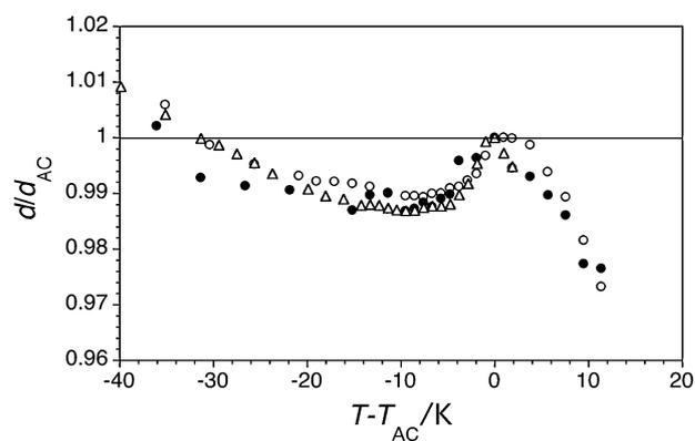
**Fig. 1** Relative smectic layer spacing  $d/d_{AC}$  versus reduced temperature  $T - T_{AC}$  for compounds **1** (●), **2** (○) and **3** (△). Data for **1** are from ref. 15.
