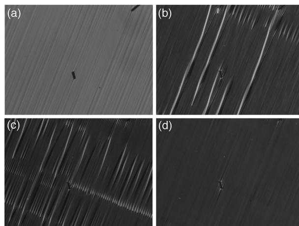
**Fig. 2** Polarized photomicrographs (400×) of a 5 μm film of **3** doped with a chiral additive (1 mol%)<sup>23</sup> in an ITO glass cell with rubbed Nylon alignment layers. The film is cooled at 10 K min<sup>-1</sup> while applying a 10 V dc field across the cell: (a)  $T - T_{AC} = +1$  K, (b)  $T - T_{AC} = -15$  K, (c)  $T - T_{AC} = -25$  K and (d)  $T - T_{AC} = -32$  K.
