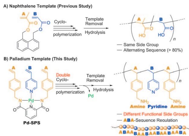
**Scheme 1.** Sequence-regulated radical polymerizations using a Pd-templated monomer.
