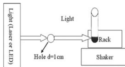
**Figure 2.** Reaction schematic figure. The samples in the reaction vessel were put on the rack which was fixed on the shaker and were irradiated by laser or LED through the wall of reaction vessel.
