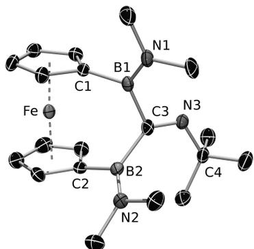
**Figure 2.** Molecular structure of **9**. Hydrogen atoms are omitted for clarity. Thermal ellipsoids represent 50% probability. Selected bond lengths (Å) and angles (deg): C1–B1 = 1.582(5), C2–B2 = 1.569(5), B1–N1 = 1.386(4), B2–N2 = 1.387(5), B1–C3 = 1.597(5), B2–C3 = 1.606(5), C3–N3 = 1.291(4), N3–C4 = 1.478(4); C1–B1–C3 = 117.3(3), C2–B2–C3 = 116.6(3), B1–C3–B2 = 111.5(3), B1–C3–N3 = 115.7(3), B2–C3–N3 = 132.7(3), C3–N3–C4 = 123.9(3),  $\alpha = 5.4$ ,  $\delta = 176.2$  (see text).
