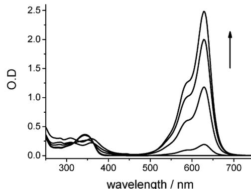
**Fig. 2** Absorption changes of **1c** (20 μM, DCM) with addition of FeCl<sub>3</sub> (0, 13, 40, 100 μM, DCM).
