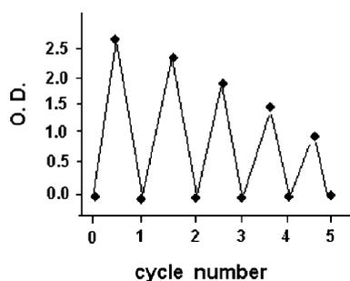
Fig. 5 Cycle number of coloration and decoloration with  $\text{FeCl}_3$  and DEA trigger in solution.
