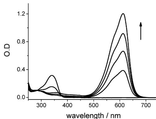
Fig. 7 Absorption changes of  $\mathbf{1c}$  (20  $\mu\text{M}$ ,  $\text{CH}_3\text{CN}$ ) with addition of  $\text{BF}_3 \text{Et}_2\text{O}$  (0, 66, 106, 160, 213  $\mu\text{M}$ ,  $\text{CH}_3\text{CN}$ ).
