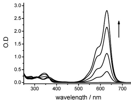
Fig. 6 Absorption changes of  $\mathbf{1c}$  (20  $\mu\text{M}$ , DCM) with addition of  $\text{AlCl}_3$  (0, 40, 80, 160, 240  $\mu\text{M}$ , DCM).
