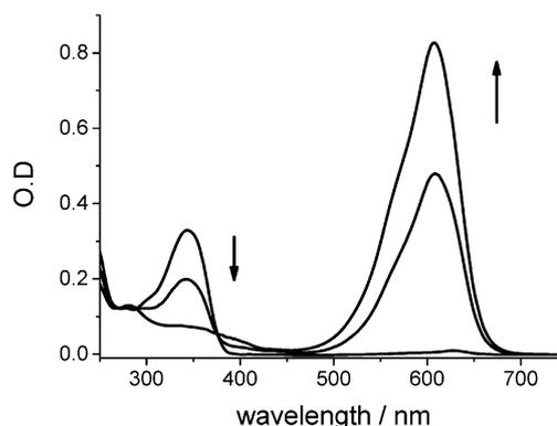
**Fig. 1** Absorption changes of **1c** (20 μM, DCM) with 365 nm light irradiation (periods: 0, 10, 20 s).
