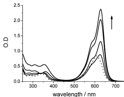
**Fig. 3** Absorption changes of **1o** (dot) with addition of FeCl<sub>3</sub> (solid) (13, 25, 50, 100 μM, DCM).
