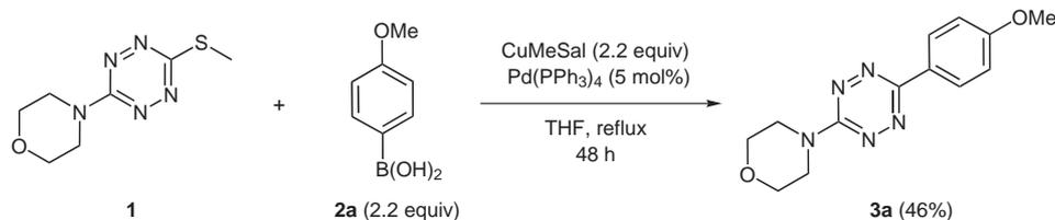
**Scheme 2** Pd-catalyzed cross-coupling reaction between tetrazine **1** and boronic acid **2a**
