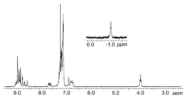
Figure 5. <sup>1</sup>H NMR spectrum of heteronuclear dimeric phthalocyanine **9c**.
