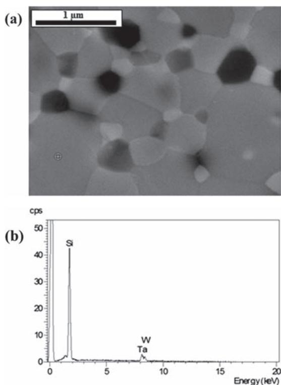
**Figure 4.** FE-SEM image and EDS of sintered TaSi<sub>2</sub>-WSi<sub>2</sub> composites.
