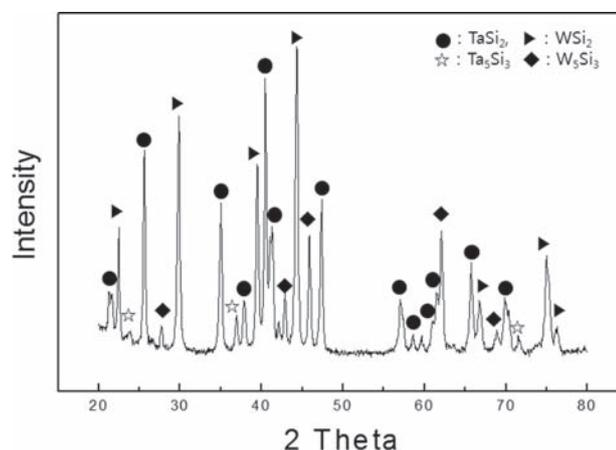
**Figure 2.** XRD patterns of the specimen sintered at 1200 °C from milled 0.5Ta-0.5W-2Si powders.
