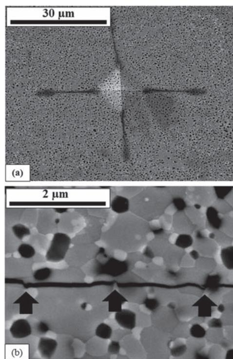
**Figure 5.** (a) Vickers hardness indentation and (b) median crack propagating in TaSi<sub>2</sub>-WSi<sub>2</sub> composites.
