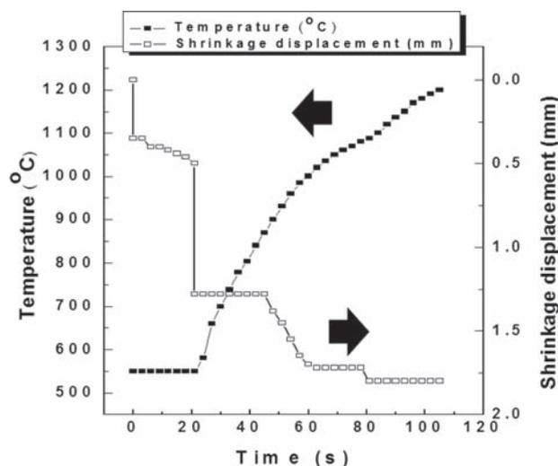
**Figure 1.** Variations of temperature and shrinkage displacement with heating time during synthesis and densification of TaSi<sub>2</sub>-WSi<sub>2</sub>.
