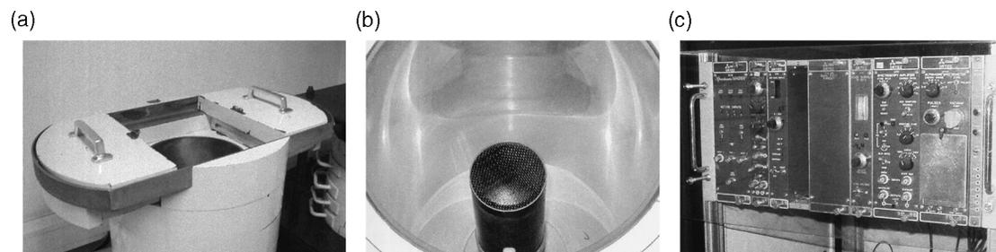
Figure 1. Gamma spectrometry equipment; 73% n-type HPGe detector with carbon window for low energy  $\gamma$  ray measurement; power supply.
