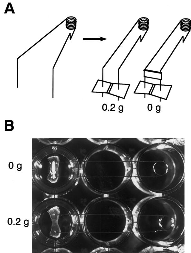
**FIG. 1.** Application of tensile stress to calvarial sutures in culture. (A) Schematic illustration of the helical springs used. See text for details. (B) Calvarial suture was removed from mice and tensile stress was applied as illustrated. The suture was suspended in the medium of each well.
