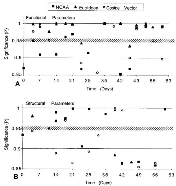
Fig. 5. Plots of significance over time of the Euclidean distance, cosine of the vector, and nonmetric clustering and association analysis (NCAA) multivariate analyses for both the functional (A) and structural parameters (B). Points above the 0.95 probability level are considered clusters significantly associated with a treatment group.
