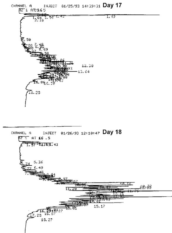
Fig. 1. Gas chromatography results from the 25- $\mu$ l treatment group on days 17 (January 25, 1993) and 18 (January 26, 1993). Day 17 was taken prior to sampling on day 18. The increase in concentrations of the Jet-A components is apparent after the stirring during the sampling of the organisms.
