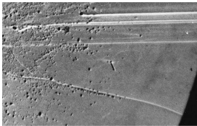
FIG. 3. (a) X-ray diffraction topograph of major area of (0001) SiC wafer: Lang method in Bragg geometry, 10 \bar{1} .10, Cu K \alpha , Bragg angle 35.8° (5 \times ). (b) Higher magnification image: Lang method in Bragg geometry, 10 \bar{1} .10, Cu K \alpha (12 \times ). The contrast is inverted to the original image.
