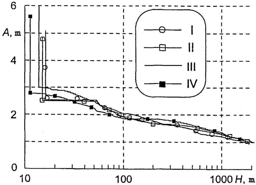
Figure 3. Variation of the height of a long wave ( $\lambda = 30$  km,  $a_0 = 1$  m) in the course of its propagation to the coast along sections I–IV in the Black-Sea Depression.
