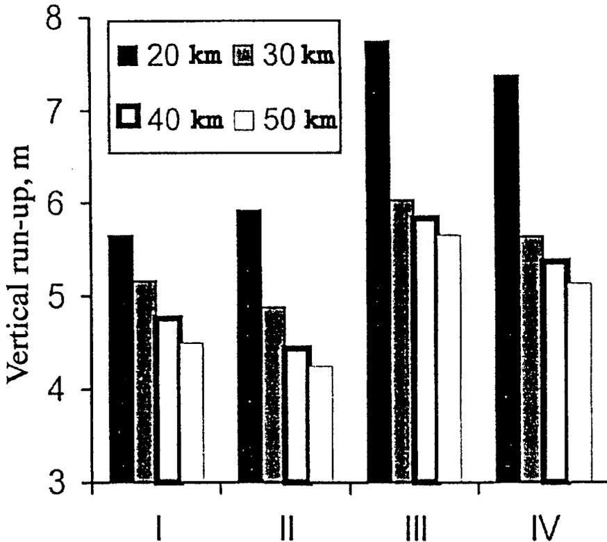
Figure 4. Run-ups of tsunami waves with initial wavelengths  $\lambda$  of 20, 30, 40, and 50 km and height  $a_0 = 1$  m on the vertical wall for the bottom profiles I-IV.
