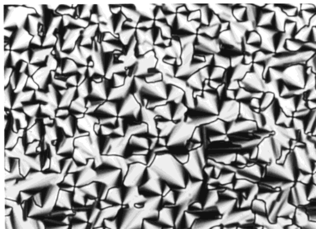
Figure 2. Photomicrograph of the Hex phase of ANBC-26 at 458.8 K, at which the CubII phase should appear on DSC because the temperature region of the Hex phase is 462–465 K in the DSC cooling; there exists a small discrepancy with temperature.
