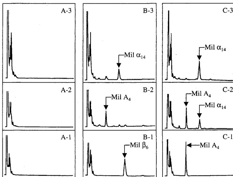
HPLC traces 1, 2 and 3 recorded 5 minutes after, 5 hours after and 24 hours after the addition of substrates, respectively.
