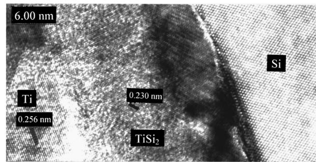
FIG. 2. High-resolution cross-sectional TEM image of a laser-annealed sample. The lattice in the middle represents that of a typical C54 phase and the lattice on the right is that of the Si substrate. Note that the silicide/Si interface is very sharp and smooth. The stoichiometry of the silicide layer is uniform and the thickness is measured to be 20 nm.
