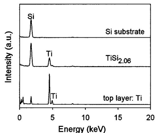
FIG. 3. EDS spectra of the layers shown in Fig. 2. The composition of the layers can be identified as (bottom) unreacted Ti with a small amount of Si (middle)  $\text{TiSi}_{2.06}$ , and (top) Si substrate.
