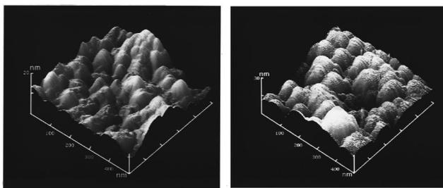
FIG. 4. AFM image of the C54  $\text{TiSi}_2$  phase produced by laser annealing (left) and RTA (right), the average grain size is measured to be 85 and 110 nm, respectively.
