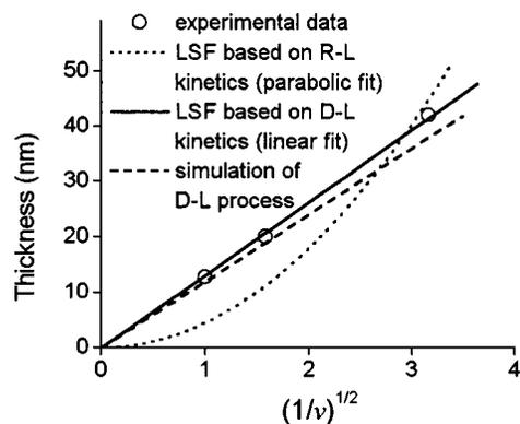
FIG. 5. Scanning speed (mm/s) dependence of silicide thickness.
