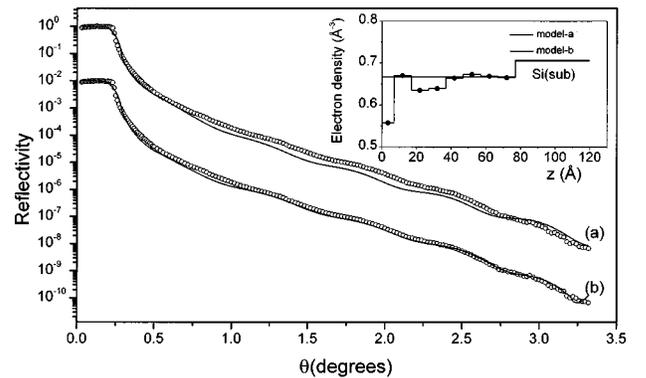
FIG. 2. X-ray reflectivity of a thermally grown SiO<sub>2</sub> film by dry oxidation process. Solid lines represent the fit using Parratt's recursion relation for model a (a), and model b (b). Inset: Electron density profiles for model a and model b. Sizes of errors are equivalent to those of symbols.
