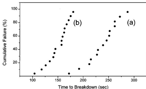
FIG. 3. TDDB plot of poly-Si/SiO<sub>2</sub>/Si(100) of thermally grown SiO<sub>2</sub> film using (a) wet oxidation and (b) dry oxidation process.
