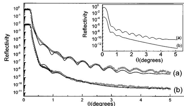
FIG. 1. X-ray reflectivity of poly-Si/SiO<sub>2</sub>/Si(100) for thermally grown SiO<sub>2</sub> films using (a) wet oxidation and (b) dry oxidation process. Solid lines represent the fitting. Inset: Simulated x-ray reflectivity curves (a) for a layer with an AED contrast of 0.01 Å<sup>-3</sup> and having smooth interfaces of 2 Å roughness, and (b) for a layer with an AED contrast of 0.06 Å<sup>-3</sup> and having both smooth and rough interfaces of 2 Å and 8 Å roughness, respectively.
