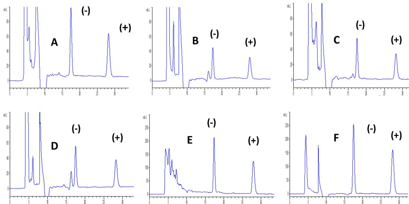
Fig. 3. Representative chromatograms of extract from five matrixes after napropamide was foliar sprayed for 5 d and standard solution of rac-napropamide: (A) extract from tomato, (B) extract from cucumber, (C) extract from cabbage, (D) extract from rape, (E) extract from soil, and (F) standard solution of rac-napropamide (50 mg/kg).
