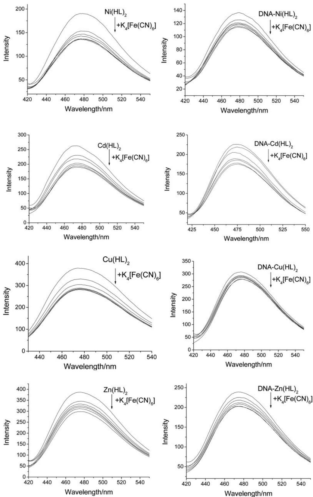
FIG. 5. Emission quenching spectra of these complexes and complex-DNA, with increasing of the concentration of the K<sub>4</sub>[Fe(CN)<sub>6</sub>] quencher.  $c_{M(HL)_2} = 1.0 \times 10^{-4}$  mol/L;  $c_{K_4[Fe(CN)_6]} = 0, 0.5, 1, 1.5, 2, 2.5,$  and  $3 \times 10^{-3}$  mol/L, and  $c_{DNA} = 40 \times 10^{-6}$  mol/L.
