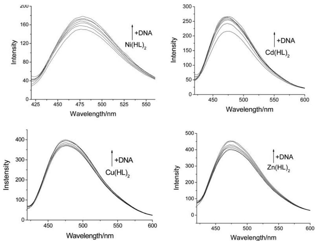
FIG. 3. The emission enhancement spectra of these complexes ( $10 \mu\text{M}$ ) in the presence of  $0, 5, 10, 15, 20, 25,$  and  $30 \mu\text{M}$  CT-DNA. The arrow indicates the emission intensity changes upon increasing DNA concentration.
