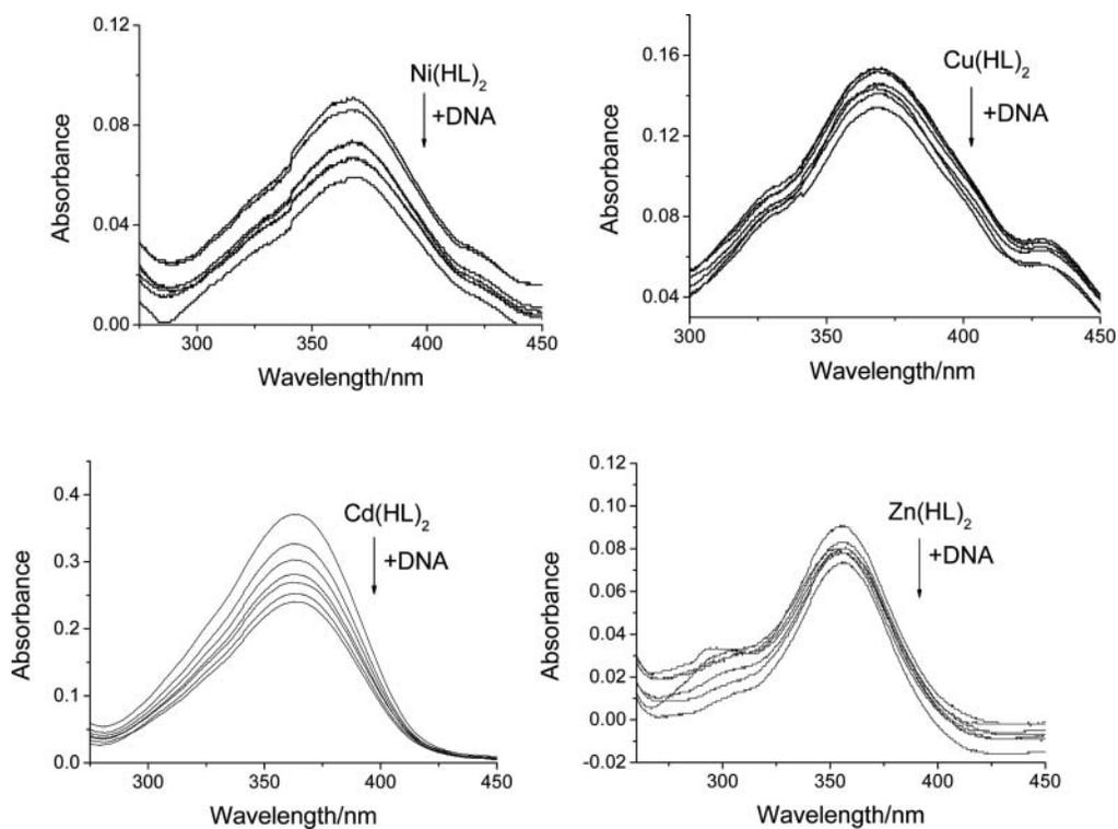
FIG. 2. Electronic spectra of these complexes ( $10 \mu\text{M}$ ) in the presence of increasing amounts of CT-DNA,  $c_{\text{DNA}} = 0, 5, 10, 15, 20, 25,$  and  $30 \mu\text{M}$ . The arrow indicates the absorbance changes upon increasing DNA concentration.
