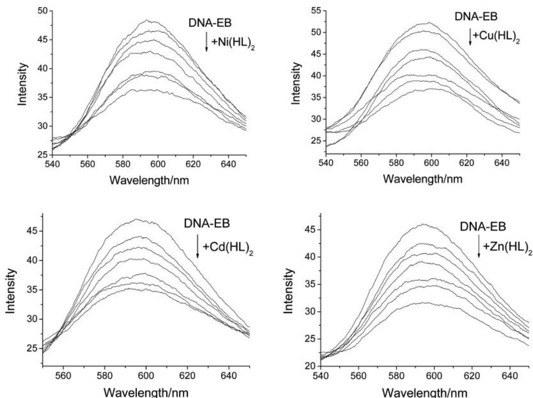
FIG. 4. The emission spectra of DNA-EB system ( $10 \mu\text{M}$  DNA and  $0.32 \mu\text{M}$  EB) in the presence of 0, 5, 10, 15, 20, 25, and  $30 \mu\text{M}$  these complexes. The arrow indicates the emission intensity changes upon increasing complex concentration.
