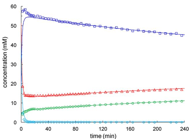
**Figure 2.** Conversion of Me(PhS)CuLi–DEF complex **2b** ( $\square$ ) to  $\text{Me}_2\text{CuLi}$ –DEF complex **3b** ( $\circ$ ). Substrate ( $\triangle$ ) and mixed cuprate ( $\diamond$ ) data are also plotted. The continuous curves are calculated by a least-squares method (see text).
