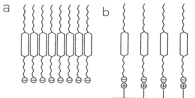
Fig. 3. The schematic representation of the 8A3 monolayer on pure water (a) and on the protonated PAA cations (b). The cross section of the molecule is determined by the molecule itself (a) and the water-soluble polymer used (b).
