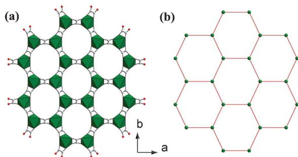
**Fig. 2** (a) The layered structure of **2** with 12-ring windows delimited by six CoO<sub>6</sub> octahedra and six oxalate ligands. (b) The compound has a hcb topology by regarding Co atoms as 3-connected nodes in the network. Color code: CoO<sub>6</sub> octahedra, green; C, gray; O, red.
