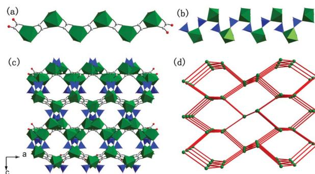
**Fig. 3** (a) Manganese oxalate chain. (b) Manganese phosphate chain. (c) The framework structure of **3** viewed along the [010] direction. (d) Compound **3** has a diamond topology by regarding Mn atoms as 4-connected nodes in the network. Color code: MnO<sub>6</sub> octahedra, green; PO<sub>4</sub> tetrahedra, blue; C, gray; O, red.
