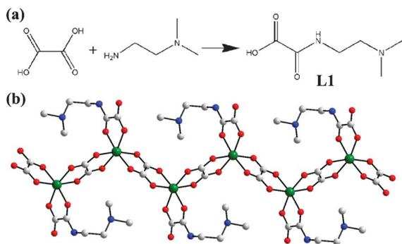
**Fig. 4** (a) Representation of the *in situ* formation of L1 ligand in compound **4**. (b) The chain-like structure of compound **4**. Color code: Zn, green; C, gray; O, red, N, blue.
