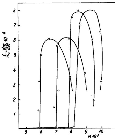
Fig. 3. Differential distribution curves for colored PEGT (from 0.1% tricrosol solution): (O) dye (b), concentration in reaction mixture 0.5%; (□) dye (b), concentration in reaction mixture 0.25%; (Δ) dye (a), concentration in reaction mixture 0.5%; (+) dye (a), concentration in reaction mixture 0.25%.
