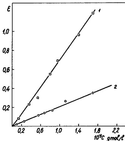
Fig. 2. Standard calibration curves for dyes in tricresol: (□) dye (a), concentration  $1.7 \times 10^{-5}$  gmole/l. in red filter; (○) dye (b), concentration  $3.4 \times 10^{-5}$  gmole/l. in red filter.
