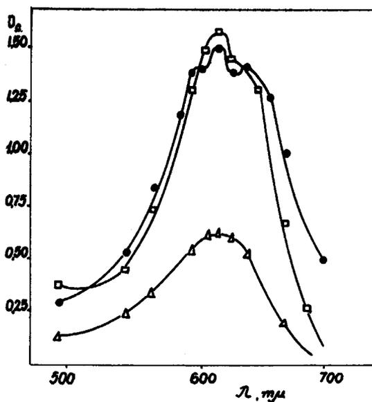
Fig. 1. Absorption spectra for dye (a) and colored PEGT (solution in tricresol): (□) pure dye (a), concentration  $4 \cdot 10^{-2}$  g/l.; (●) pure dye (a), heated, concentration  $4 \cdot 10^{-2}$  g/l.; (Δ) colored PEGT, concentration  $8 \cdot 10^{-2}$  g/l.
