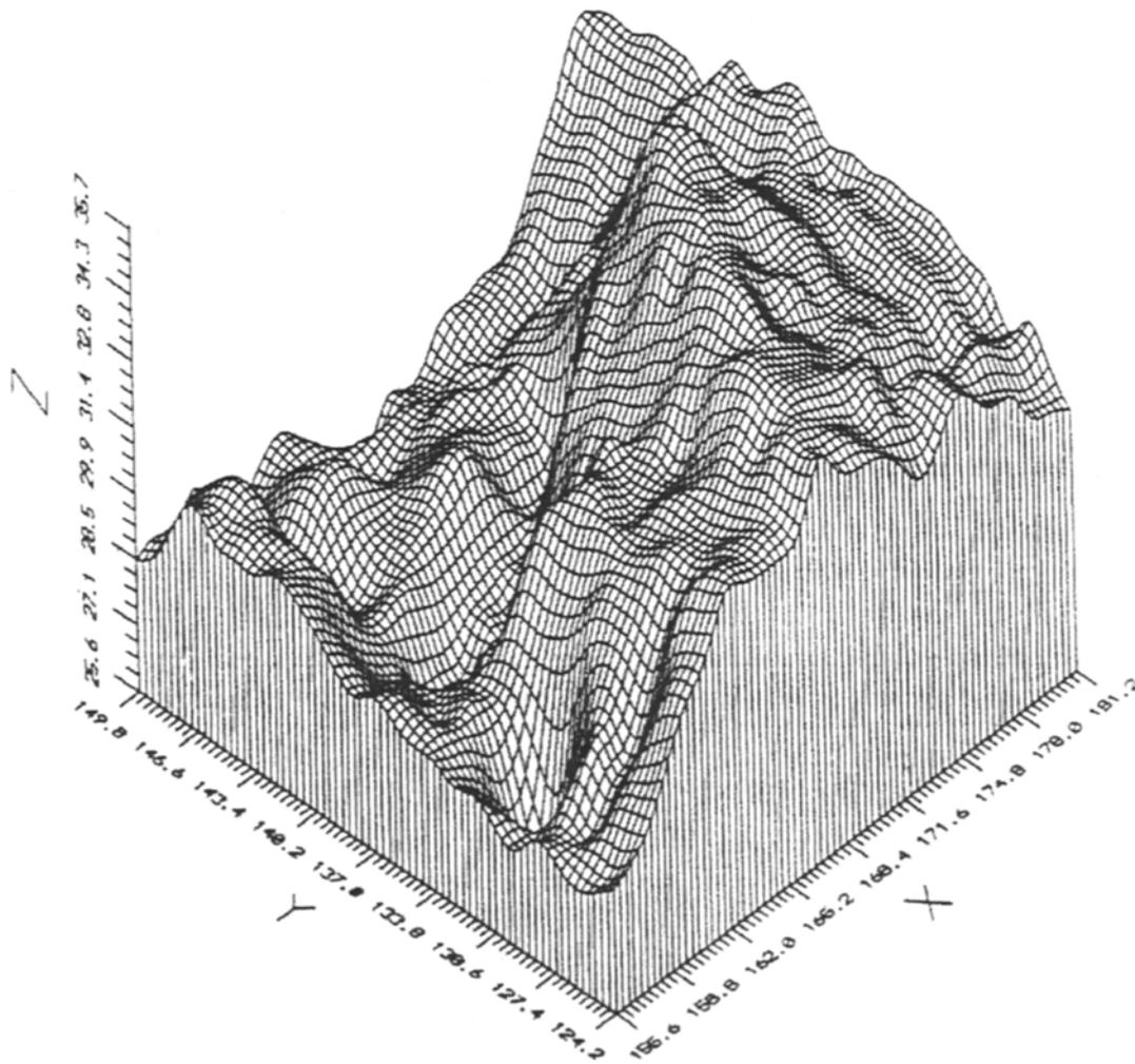
**Fig. 2.** Perspective projection of a stepwise brittle-fracture surface.
