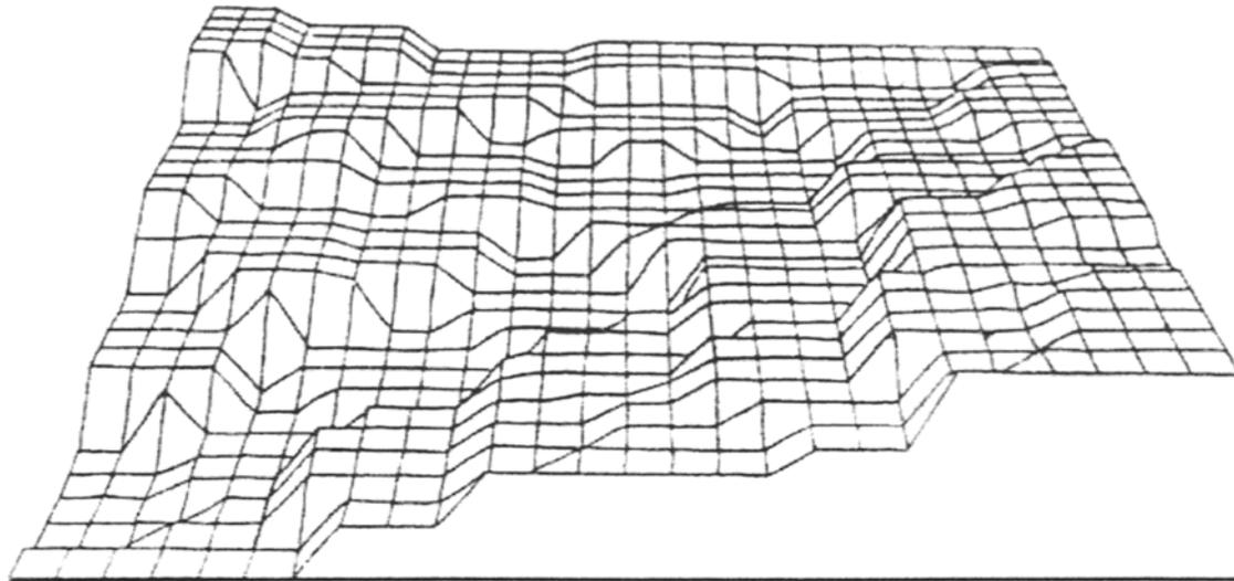
**Fig. 1.** Digital model of a micropattern of the fracture surface plotted by the method of extrapolation of the data of stereoscopic measurements in scanning electron microscopy.
