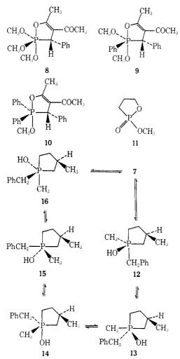
sented by Whitesides and Bunting which strongly suggests that apical-equatorial interchange and racemization share a common mechanism.<sup>20</sup> Since structures 7, 12, and 13 should produce the *trans* oxide and 14–16 the *cis* oxide, both 1a and 1b would be expected to lead to *mixtures* of the *cis* and *trans* oxides 2a and 2b if pseudorotation of 7 were operative.
