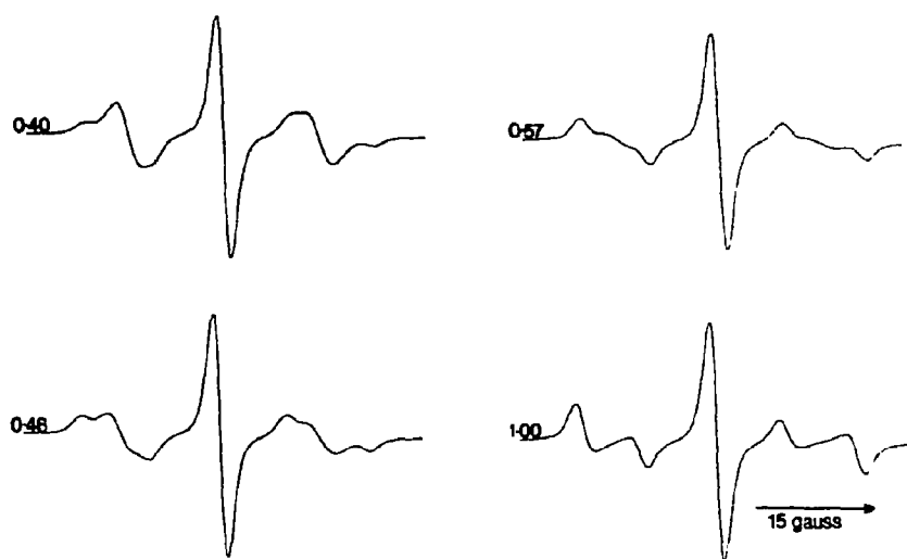
Fig. 2. Simulated spectra obtained with the elliptical distribution function given by eq. (7); each spectrum is labelled with the value of the ratio b/a .
