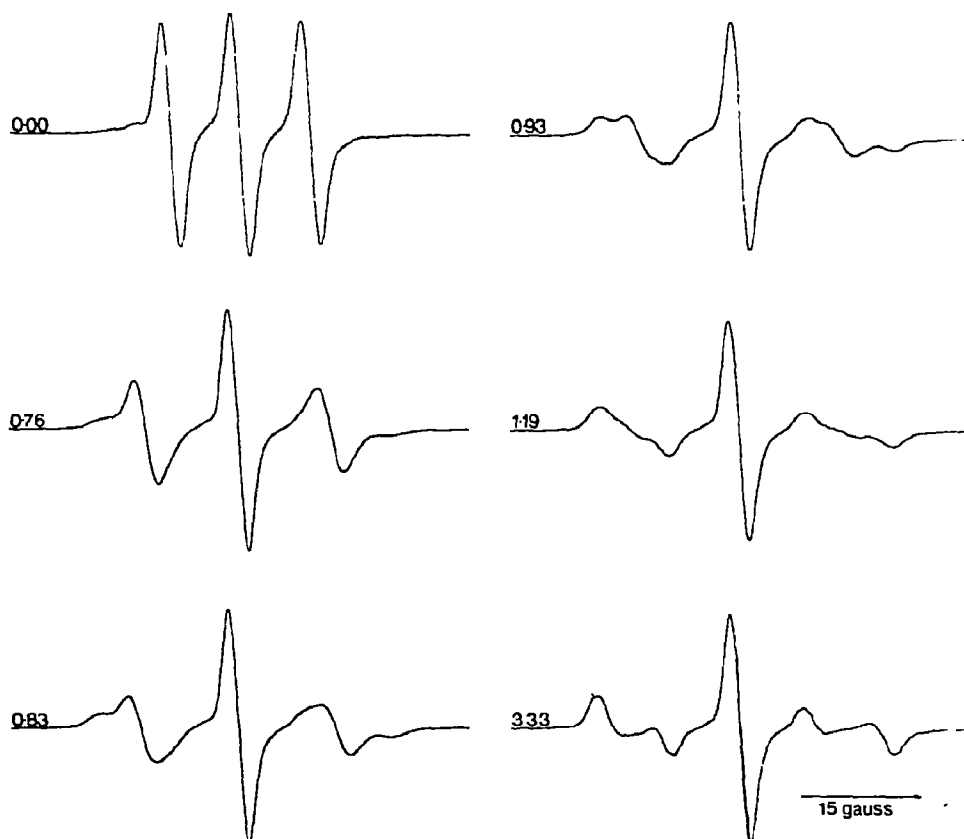
Fig. 1. The electron resonance spectra for the spin probe dissolved in the nematic mesophase of 4,4'-dimethoxyazoxybenzene measured as a function of the angular velocity; the number associated with each spectrum is the spinning speed in Hz.
